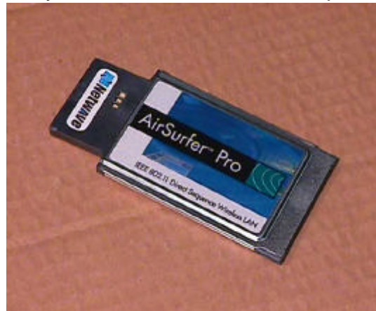
Figure 1. Baystack 660 series wireless PC card (Netwave version shown).
