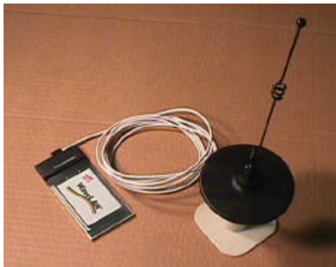
Figure 3. WaveLAN PC card with external antenna
